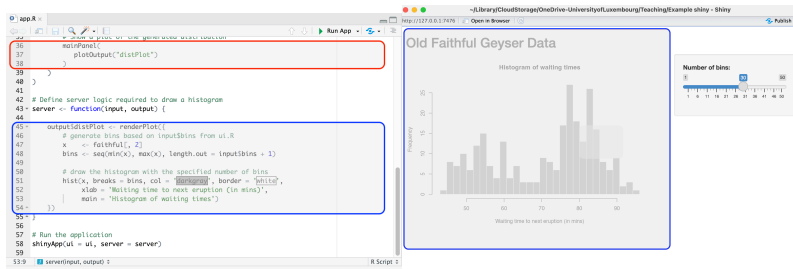
(a) UI code and corresponding server code for output object. (b) Corresponding plot display in the user interface.
